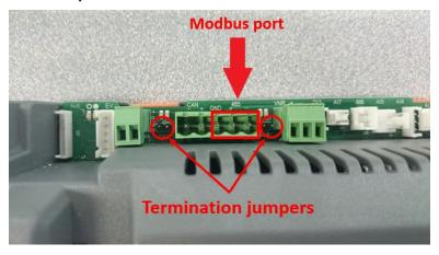
Figure 10: Modbus port and termination jumpers
