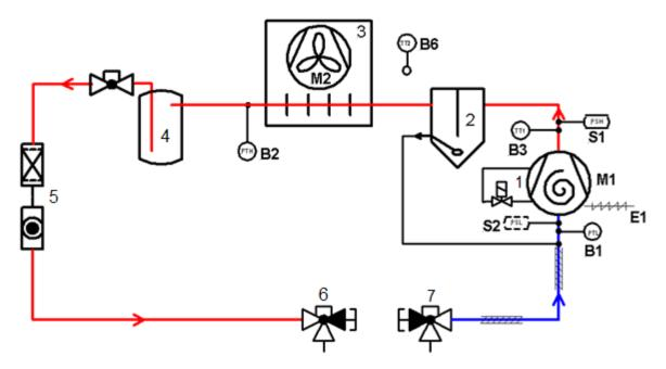
Figure 6: P&I diagram for ZXDE units
