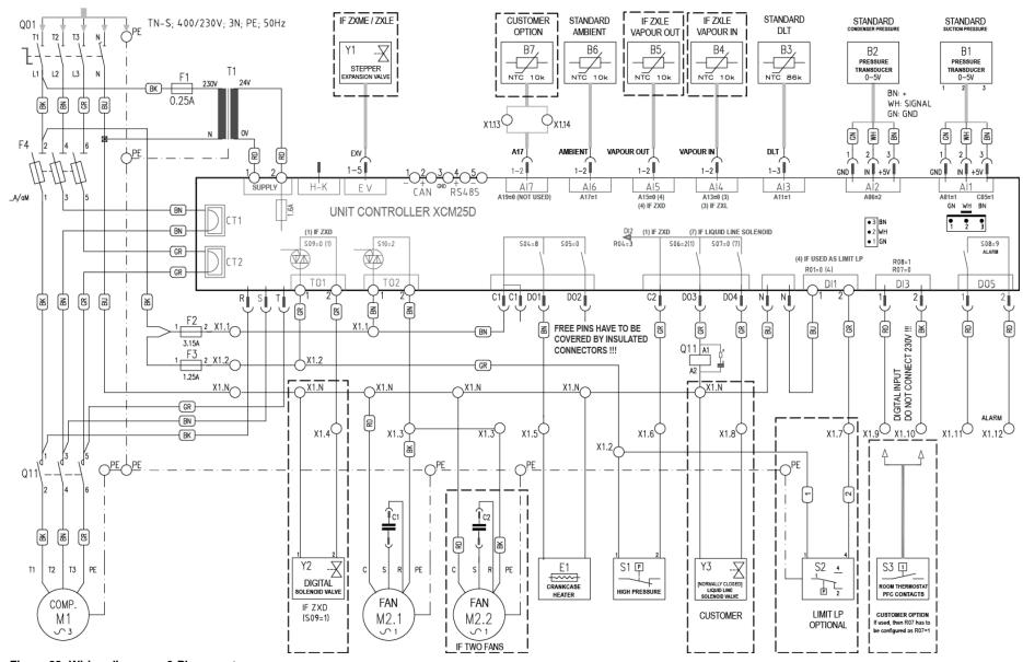
Figure 28: Wiring diagram - 3-Phase motor
