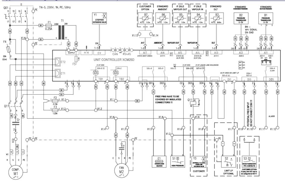
Figure 29: Wiring diagram – 1-Phase motor
