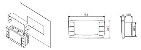
Figure 14: Remote display front panel mounting
