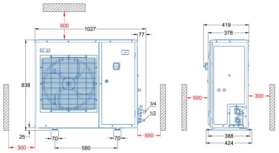
Figure 24: Fixing dimensions and distances - Single-fan units
