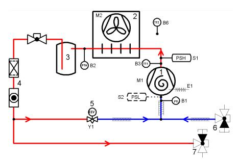
Figure 4: P&I diagram for ZXME units
