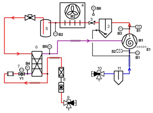
Figure 5: P&I diagram for ZXLE units
