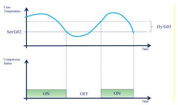
Figure 12: External temperature sensor - Functionality
