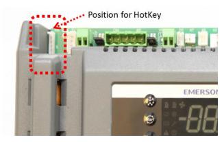
Figure 19: Location of "Hot Key" plug connection
