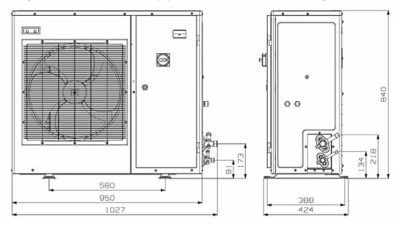
Figure 1: Dimensions of models ZXME020E to ZXME040E, ZXDE030E and ZXLE020E to ZXLE040E (single-fan units)
