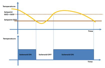
Figure 17: Pumpdown functionality with temperature sensor
