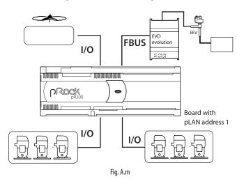
Cascade, 2 suction lines, 2 condenser lines (built-in driver for managing the heat exchanger on the second line), single board;
