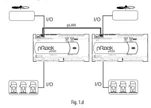
**Example 5**: 2 suction lines on separate boards with scroll or piston compressors, 2 high pressure line on separate boar
