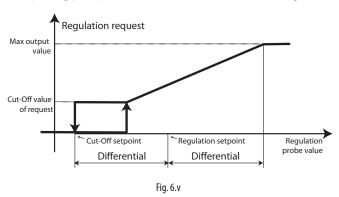
A percentage of the control request and a cut-off set point can be set. When the control request reaches the set cut-off value, this value is kept constant until the control value falls below the cut-off set point, after which it falls to 0 % and remains there until the request exceeds the cut-off value again.
