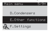
The top right corner shows the selected item and the current password level (for details see the following paragraph). The  $\uparrow$  and  $\checkmark$  buttons are used to select the desired menu item, while  $\hookleftarrow$  accesses the selected item.
