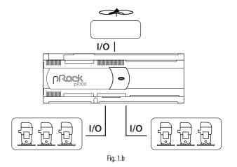
**Example 4:** 2 suction lines on board (scroll or piston compressors), 2 high pressure lines on the board):
