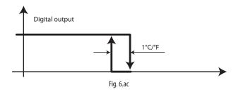
In the second case, the output is active for liquid temperature values greater than a threshold, with fixed differential.
