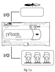
**Example 2**: 2 suction lines on the same board with scroll or piston compressors, 1 high pressure line:
