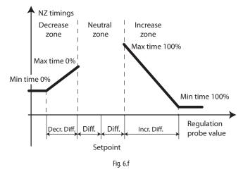
As well as the decrease and increase differentials, 4 times need to be set, two for each zone, which represent the maximum and minimum time to reach the request, equal to 0% or 100%, for the decrease and increase respectively.
