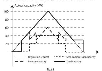
**Example** 2: range of modulating device capacity variation lower than the capacity of the compressors: two compressors without capacity control, with the same capacity, 30 kW each, modulating device with variable capacity between 20 and 40 kW.
