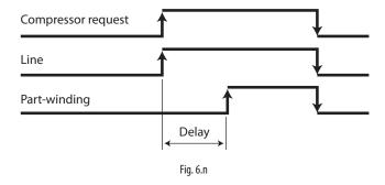
For star/delta starting, the star time, the delay between the activation of the line and star digital input, and between the delta and star digital input all need to be set, as shown in the figure:
