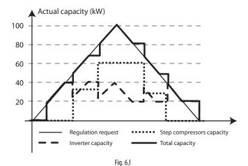
Esempio 3: range of modulating device capacity variation in between the capacity of the compressors, all different sizes: two compressors without capacity control, capacities 15 kW and 25 kW, modulating device with variable capacity between 10 and 30 kW.
