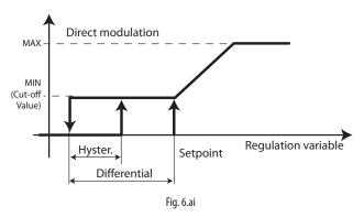
If an enabling variable has been set, the corresponding output is active if the enabling is also active. For each modulation, a high alarm threshold and a low alarm threshold can be set, and are absolute. For each alarm, the activation delay and priority can be set. See chapter 8 for details on the alarms. For modulation a minimum and maximum value can also be set for the output, and the cut-off function can be enabled, with operation as shown in the previous figure.
