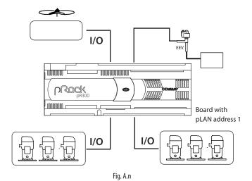
Cascade, 2 suction lines, 2 condenser lines (built-in driver for managing the heat exchanger on the second line), double board;
