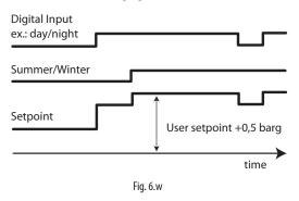
Note: the same digital input is used for set point compensation on each line, so if suction and condensing pressure set point compensation is activated by digital input, both compensation functions are active at the same time.
