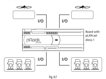
g. 2 suction lines on the same board (scroll or piston compressors), 2 condenser lines on separate boards:
