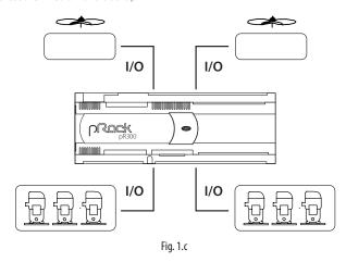
**Example 4:** 2 suction lines on separate boards (scroll or piston compressors), 2 high pressure lines (on the first suction line board):
