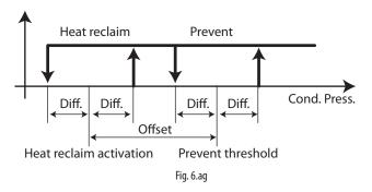
The function must be enabled and an offset must be set in relation to prevent threshold, while the differential is the same set for the prevent function.
