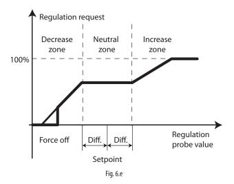
Inside the neutral zone the capacity request sent by the controller is constant (except when there is a modulation device and modulation is enabled inside the neutral zone, as described in the following paragraph) and the value satisfies the temperature control request in those specific operating conditions, therefore within this zone no device is stopped or started.
