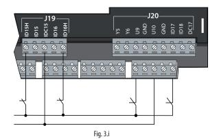
3.4.8 Remote connection of the digital inputs
