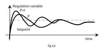
The integral action depends on the time and the deviation from the set point. This modifies the request if the control value does not approach the set point for some time.
