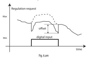
By suitably setting this parameter based on system configuration, one compressor can be shut down; for example if there are three compressors, by setting the decrease to 33%, activation of the input stops one of the three compressors. Compressor shutdown and restart respect the safety times.
