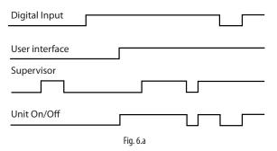
When there are two suction and condenser lines, on-off is independent for each line, while when there are two suction lines and one condenser line, it is independent for the suction lines, while the condenser line stops when both suction lines are off, and starts when at least one suction line is on.
