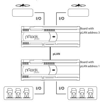
h. 2 suction lines on separate boards (scroll or piston compressors), 2 condenser lines (one for each suction line board)
