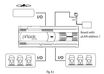
Pumped, 2 suction lines (external driver for managing the heat exchanger on the first line), 1 condenser line, double board
