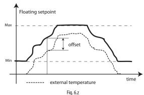
Note: if set point compensation from scheduler, digital input or supervisor is also active, the offset is added to the minimum and maximum limits for the floating set point.
