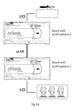
2 suction lines on the same board (scroll or piston compressors) and up to 1 condenser line:
