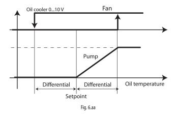
If a digital output and just one pump is used, the fan and the pump are activated/deactivated at the same time:
