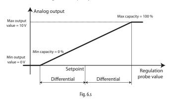
Example 2: minimum modulating output value 0 V, maximum value 10 V, minimum modulating device capacity 60 %, maximum 100 %.
