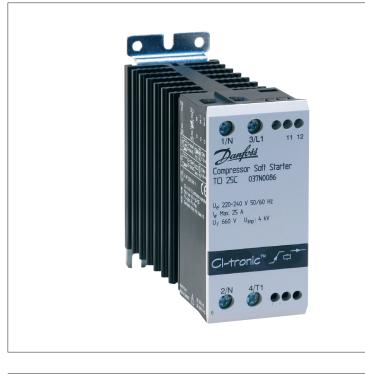
The TCI 25C soft starter is designed for soft starting of single-phase compressors. During start the TCI 25C will gradually ramp-up the motor voltage to full line voltage thus reducing the starting current peak.
