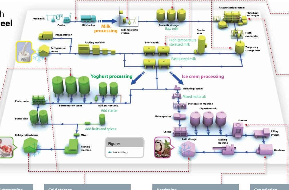
Fermentation, cooling and maturation Fermentation by lactic acid cultures and subsequent cooling
