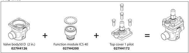
Figure 43: ICV 40 valve body w/different connections
