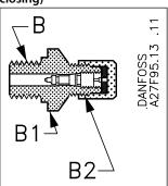
Table 53: Pressure gauge connection, 1/4 in. flare (self-closing)
