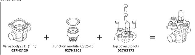
Figure 29: ICV 25 valve body
