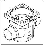
Table 32: ICV 40 valve body w/different connections
