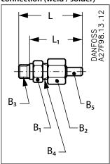
Table 51: Pressure gauge connection (weld / solder)
