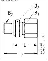
**Table 55: Pressure gauge connection (cutting ring)**
