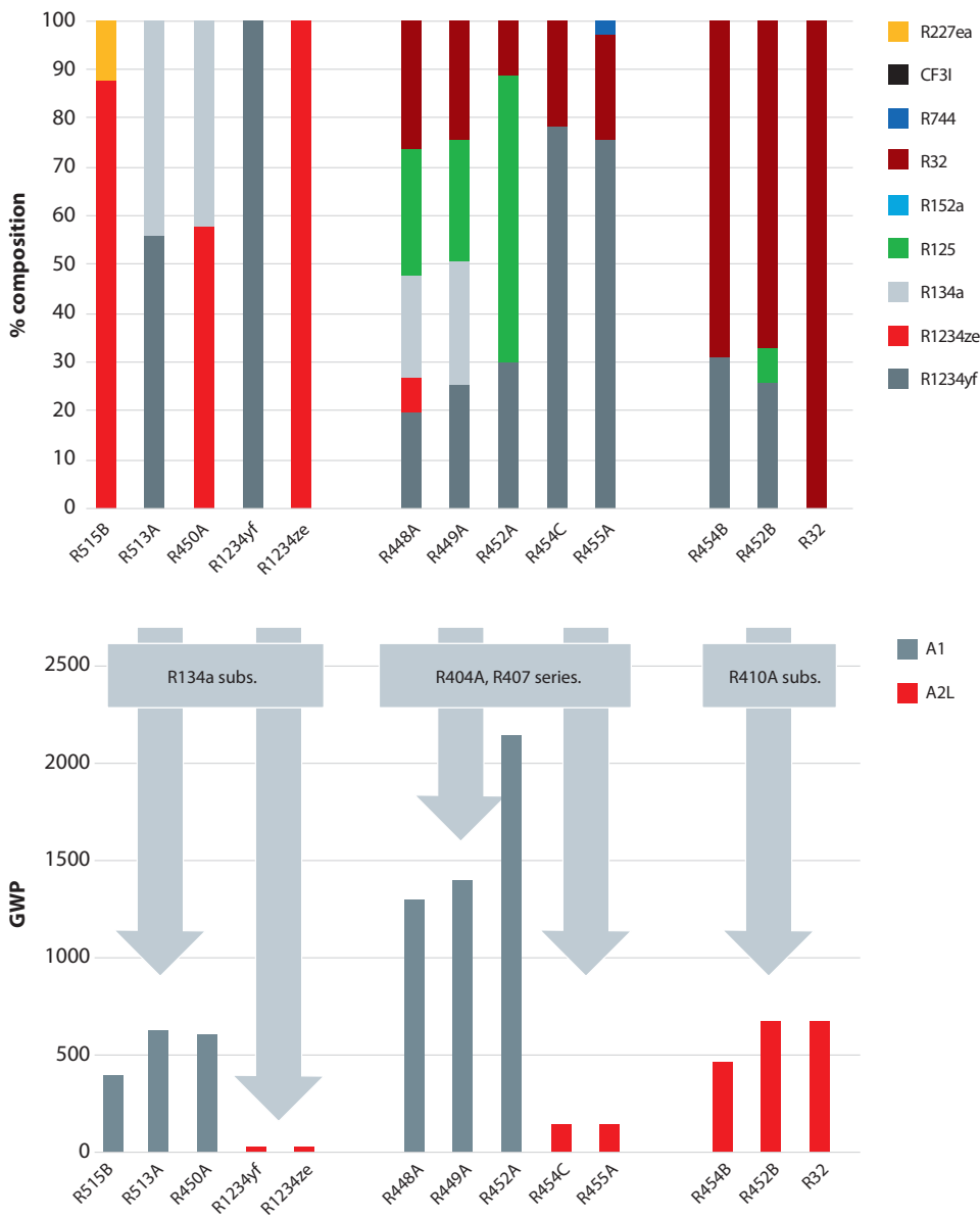
Figures 13a and 13b: The main replacement options and their composition and GWP levels
