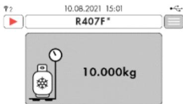
The weight value from the connected REFSCALE is displayed on this screen.
