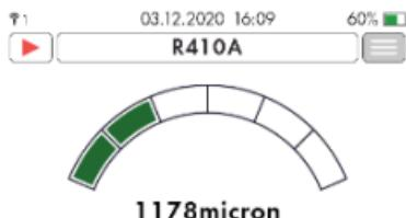
The vacuum value from the connected REFVAC-RC is displayed on this screen.
