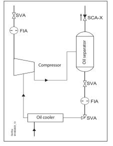
The above shows the check & stop valve SCA-X in the discharge line of a screw compressor unit. The SCA-X valve in the discharge line prevents "back condensation" in the oil separator as well as pressure equalising through the compressor.
