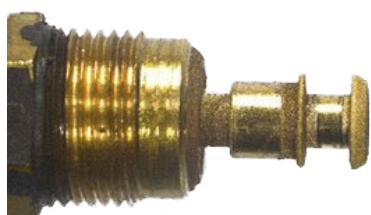
Corrosion of a solenoid valve by using a Bio30 fuel with brass material
