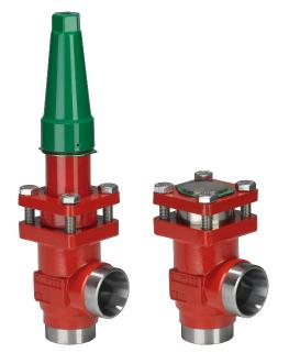
SCA-X are check valves with a built-in stop valve function. CHV-X are check valves only. SCA-X/ CHV-X are available in angleway versions. The valves are designed to open at very low differential pressures, allow favourable flow conditions and are easy to disassemble for inspection and service.
